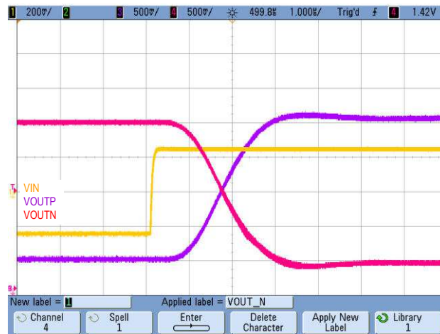
Figure 8-4. Step Response of the AMC1301
