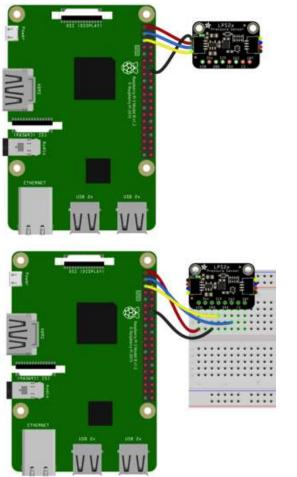
Pi 3V to sensor VCC (red wire) Pi GND to sensor GND (black wire) Pi SCL to sensor SCL (yellow wire) Pi SDA to sensor SDA (blue wire)
