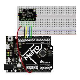
Connect Vin to the power supply, 3V or 5V is fine. Use the same voltage that the microcontroller logic is based off of Connect GND to common power/data ground Connect the SCK pin to Digital #13 but any pin can be used later Connect the SDO pin to Digital #12 but any pin can be used later Connect the SDI pin to Digital #11 but any pin can be used later Connect the CS pin Digital #10 but any pin can be used later
