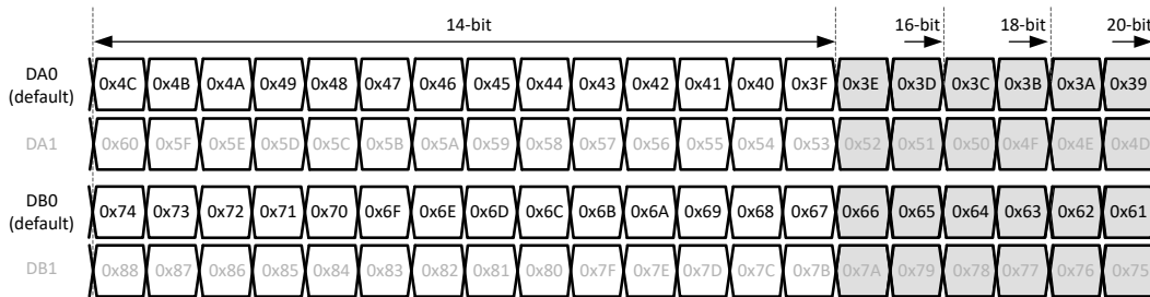
Figure 8-46. 1-wire output bit mapping
