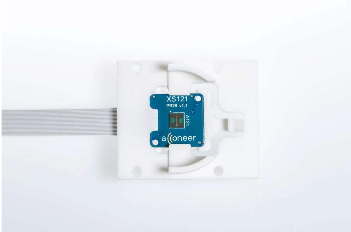
Picture 16. XS121 mounted in LH112.
