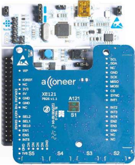
Picture 8. XE121 connected to an STM Nucleo Development Board.
