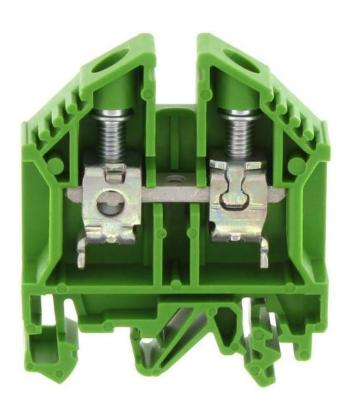
Feed-through terminal, Screw connection, Mounting type:Mounting rail TS 35/7.5 and TS 32, Rated cross-section: 16 mm², Width: 12 mm, Colour: Green
