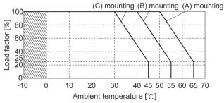
\*In case of ADA600F-24, load factor 100% means output 24V, 14A at ACIN100V, 24V, 15A at ACIN200V.
