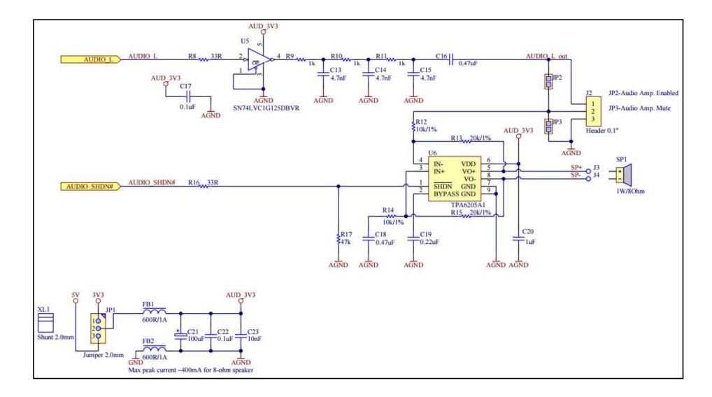
This is a reference schematic from FTDI, which can be used to successfully filter and amplify the audio signals coming from the NHD EVE2 TFT Module.
