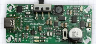
After adding the remaining components (USB Type C port, large capacitor and inductor, two switches) you are basically done with the PCB.
