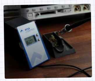
Heat up your soldering iron. Use a temperature of around 360 degrees Celsius for most of the SMD solder connections. You will notice though that some solder joints will be harder to create due to the heat absorption by the copper mass that forms the GND layer. There you can use 400 degrees Celsius.
