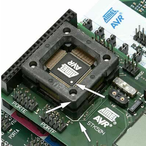
Figure 3-3: Placing the AVR in the ZIF socket
