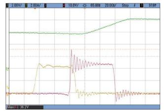
Figure 4: Typical Waveforms for V<sub>IN</sub> = 24 V to 1.2 V/7 A (1000kHz) Buck converter CH1: V<sub>PWM</sub> Input voltage — CH2: (Iout) Switch node current — CH4: (Vout) Switch node voltage
