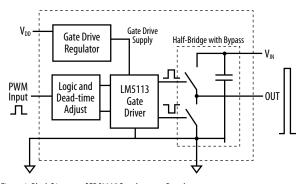
Figure 1: Block Diagram of EPC9005 Development Board
