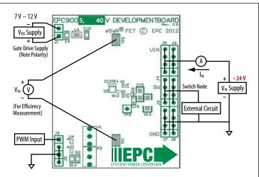
Figure 2: Proper Connection and Measurement Setup
