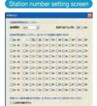
Simply tick the boxes in the "Station number setting screen" to choose measuring instruments connected via RS485.
