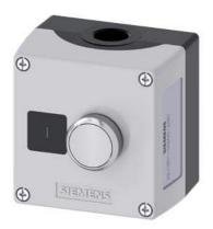
Enclosure for command devices, 22 mm, round, Enclosure material metal, enclosure top part gray, 1 control point metal, A=Pushbutton white, 1 NO, screw terminal, floor mounting, label: I, 1xM20 each on top and bottom, Label enclosed
