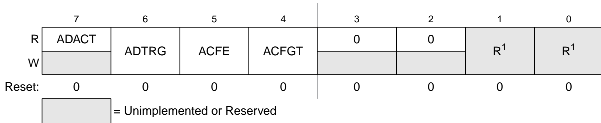
Figure 9-5. Status and Control Register 2 (ADCSC2)
