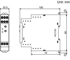
\*Installation Procedure: Mount to the DIN Rail or with front screws \*Dimensions for Mounting with Front Screws
