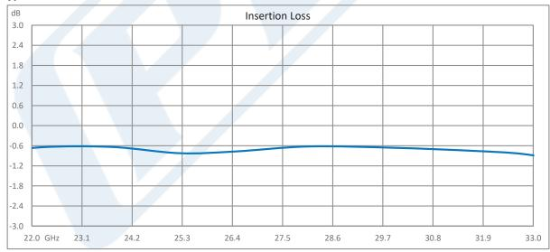
Click the following link (or enter part number in "SEARCH" on website) to obtain additional part information including price, inventory and certifications: Isolator with 13 dB Isolation from 22 GHz to 33 GHz, 10 Watts and 2.92mm Female PE83IR1035
