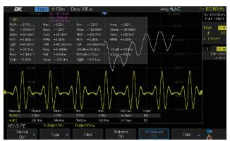
Display 36 automated measurements that include voltage, time, and statistics. Arithmetic and FFT functions can be performed on analog channels and two reference signals.
