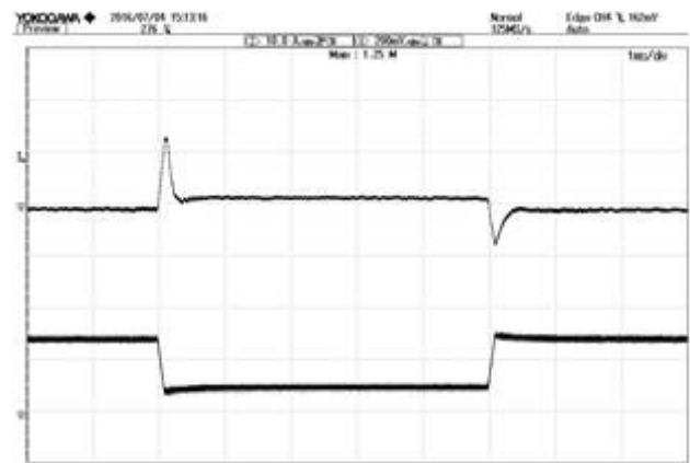
Figure 2: V_{out} vs. V_{in} @ Full load
