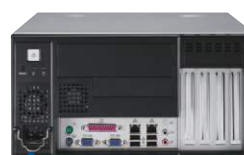
Plug ring-lock securely fastens the power cord
