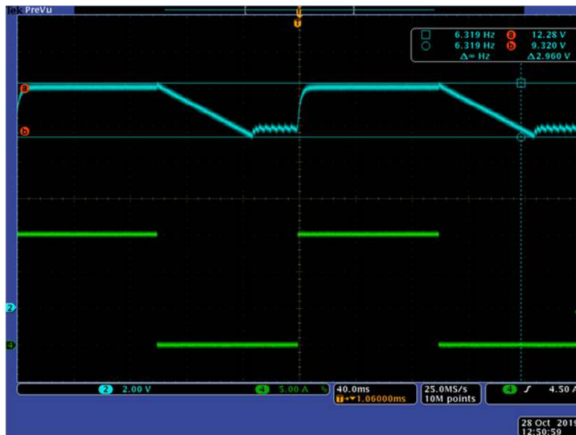
Figure 20. 10 mA to 15 A Transient (Ch2 = V_{OUT} DC Coupled; Ch4 = I_{OUT} )
