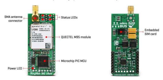
There are four LEDs used to display the connection status. Before the connection and communication with the AWS is possible, the setup procedure must be followed. For detailed step by step information, refer to the setup manual.
