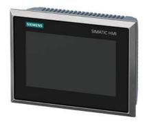
SIMATIC HMI TP700 Comfort INOX Stainless steel front, glass pane, capacitive touch, degree of protection front IP69K, 7" widescreen TFT display, PROFINET interface, MPI/PROFIBUS DP interface, 12 MB configuration memory, Windows CE 6.0, WinCC Comfort V15.1
