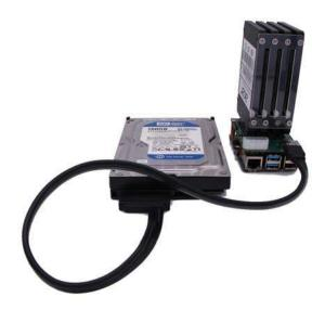
The Penta SATA HAT is powered by the JMB585 with 2 5Gbs PCIe buses with up to 10Gbps bandwidth. With 5 SSD's configured in Raid0 mode, an archiving speed of up to 803MB/s can be achieved.
