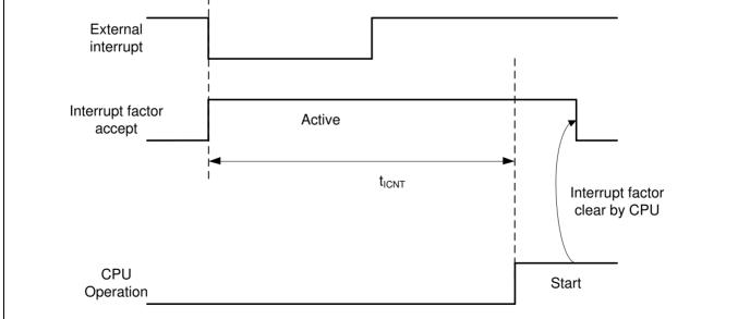
$<sup>^{71}</sup>$  The maximum value depends on the condition of environment.  $^{72}$  toscwr: Oscillator stabilization time.  $^{73}$  External interrupt is set to detecting fall edge.
