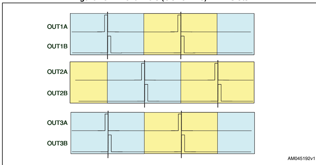
Figure 28. 2.1 channels (OCFG = 10) PWM slots
