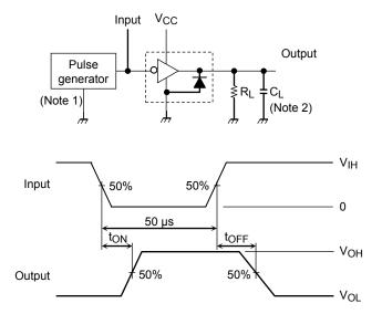
Note 1: Pulse width 50  $\mu$ s, Duty cycle 10% Output impedance 50  $\Omega$ ,  $t_r \le 5$  ns,  $t_f \le 10$  ns,  $V_{IH} = 5.0$  V
