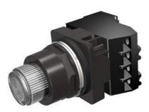
30mm BlackMax, Epoxy Coated Corrosion Resistant Complete Metal Unit PTT / Illuminated Pushbutton Transformer type, 600V AC Incandescent Lamp Extended Button Plastic Lens, Clear 2 Position Momentary with 1 N.O. - 1 N.C. Heavy Duty Contacts, A600/P600 UL Listed, CSA Certified NEMA 1,3,3R,4,4X,12,13 & Automotive Standards
