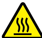
W3198 Heated/Hot Surface Hazard
