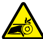
W3154 Belt Drive Entanglement Hazard
