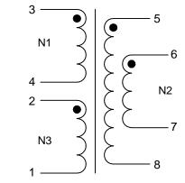
N2 denotes two windings connected in parallel. Terminals 5+6 and 7+8 must be tied as solder bridging is allowed.
