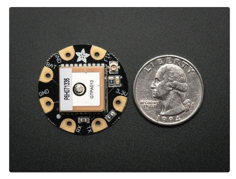
This module is the best way to add a GPS to your wearable project. Installed on the PCB is the latest of our Ultimate GPS modules, a small, super-thin, low power GPS module with built in data-logging capability! This module's easy to use, but extremely powerful. It's does not use i2c like the other sensors, but rather communicated over serial to FLORA. Use it for a GPS Jacket () of GPS logging dog harness ().
