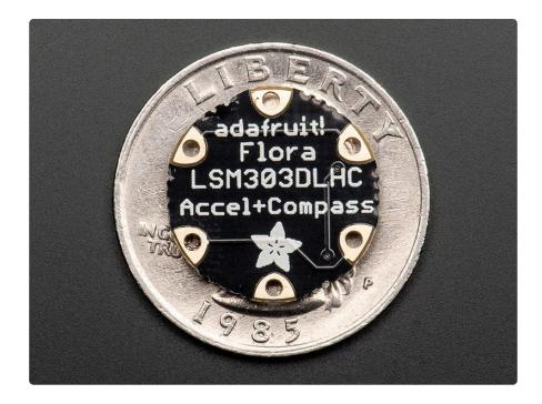
The LSM303 board also contains a compass, which you can use to tell which way you're facing. Use it alone to get your cardinal bearings, or in combination with a GPS for navigation like in the NeoGeo watch () or Citi Bike helmet ().
