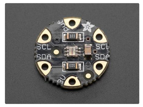
Now let's shed some light on the TSL2561 luminosity sensor. It'll read visible light, infrared, or both. Maybe you could make a darkness-activated headlamp or a hat that detects infrared security cameras.
