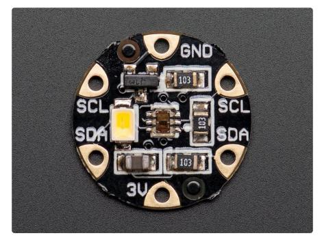
You can detect the color of an object with the TCS34725 color sensor. The onboard LED shines onto the object, reflecting light into the sensor for an accurate color reading, great for matching your accessories to your outfit like in the <u>Chameleon</u> Scarf () or FLORAbrella ().
