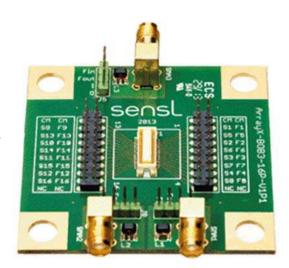
Two SMA connectors and Balun transformers are provided with 4-pin headers to allow any fast signal to be connected directly to the SMA or via the transformer using jumper wires.
