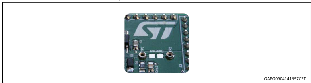
Figure 4: Mounting through-hole sense resistor
