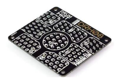
Hook up these 8 advanced capacitive touch pads with LED indicators to start making sublime beats and control surfaces with your Raspberry Pi.
