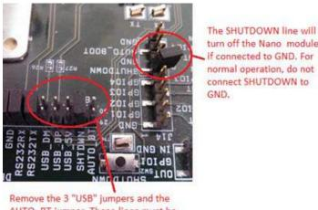
AUTO BT jumper. These lines must be disconnected for the pre-production version of the Nano module to work properly.
