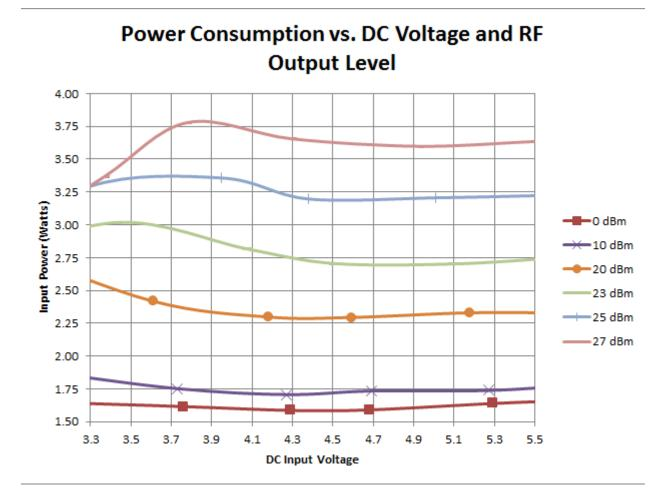
Note: Power consumption is defined for operation into a 17 dB return loss load (VSWR of 1.33) or better. Power consumption may increase, up to 4 W, during operation into return losses worse than 17 dB and high ambient temperatures. Power consumption will also vary based on which of the <u>Supported Regions</u> is in use.
