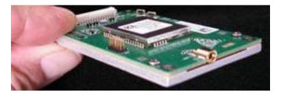
Make sure it is assembled as shown in these pictures so no live signals are shorted to ground.
