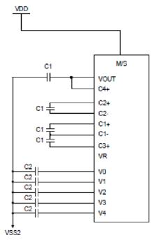
C1: 1uF-4.7uF for Voltage rating from 10-35V C2: 1uF-2.2uF for Voltage rating from 6.3-25V
