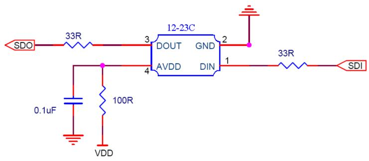
When EASV3015ICRGBA0 is set to operate on 5V power system, a 0.1uF capacitor is recommended to add between power supply and ground terminal. The capacitor is suggested to put as closer as possible to IC position. There are frequent resistors were used on different drain voltage as listed table.
