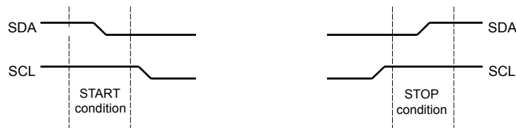
Figure 13-3. START and STOP Conditions
