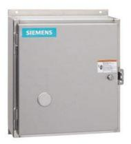
Electrically held lighting contactor, Contactor amp rating 20A, 0 N.C. / 4 N.O. Poles, 24VAC 50/60HZ coil, Non-combination type, (no disconnect device), Encl NEMA type 4X 304 S-Steel, Water/dust tight noncorrosive
