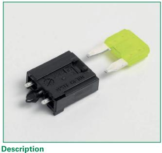
Fuse holder for MINI/ FK1 fuses for PCB applications. The FL1 Fuse Holder can be mounted in a row of nearly any number. The terminals fit into a 7.62 mm pitch.
