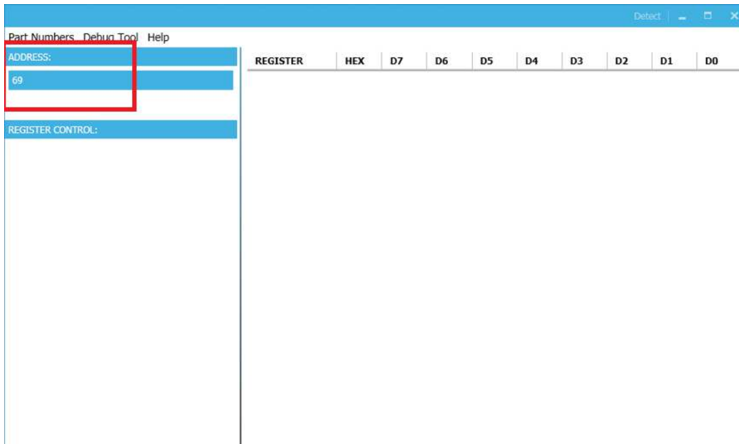
Figure 7: Appearance of Address Shows Successful Connection
