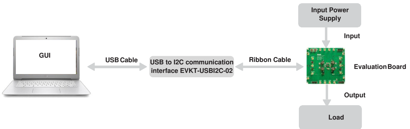
Figure 1: EVKT-5416 Evaluation Kit Set-Up
