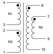
N2 denotes two windings connected in parallel. Terminals 7+8 and 9+10 must be tied as solder
