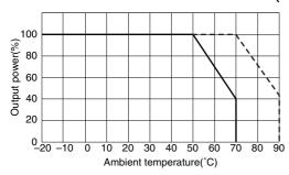
• If the case temperature is used for the derating, apply the range indicated by the dashed line.
