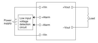
The input voltage detection output terminal ( $\pm$ Alarm) is a transistor output of a photo-coupler and it is insulated at the both input and output sides.
