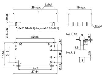
Weight: 6g Dimensions in mm Tolerance: ±0.3
