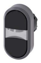
Twin pushbutton, 22 mm, round, plastic with metal front ring, black, black, pushbuttons, flat, with laser labeling, upper case and lower case, always upper case at the beginning of the word
