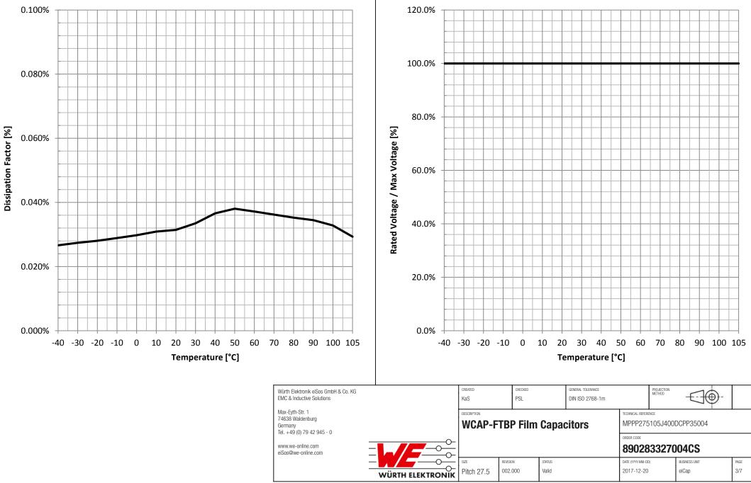
**Rated Voltage vs. Temperature:**
