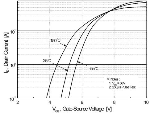
Figure 2. Transfer Characteristics
