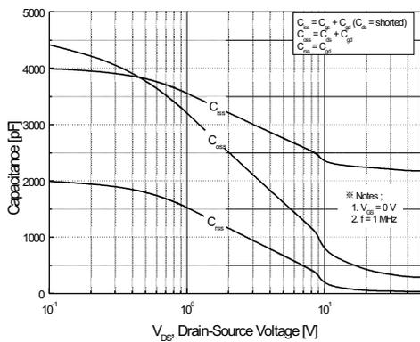
Figure 5. Capacitance Characteristics
