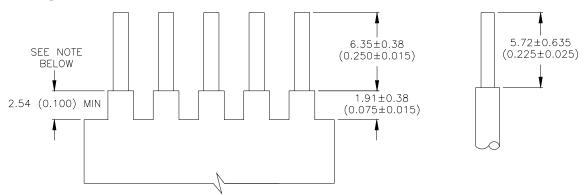
NOTE: If cable has a shield over the conductor, it should be cut off at a point not closer than 2.54 (0.100) from the end of the stripped conductor, and ground lead extended as shown in drawing for termination.
