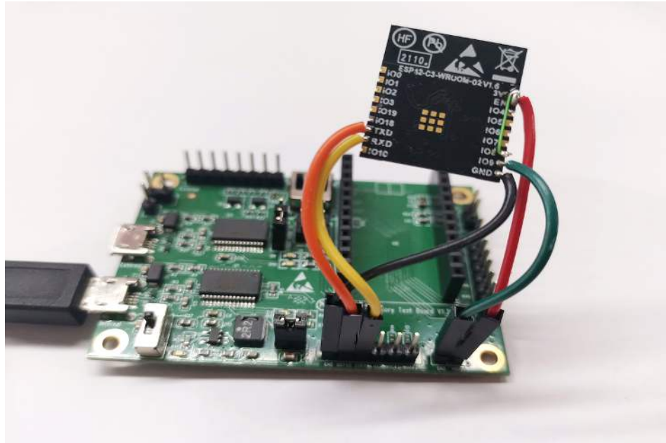
Figure 2-1. Wiring for ESP32-C3-WROOM-02 in Download Mode
