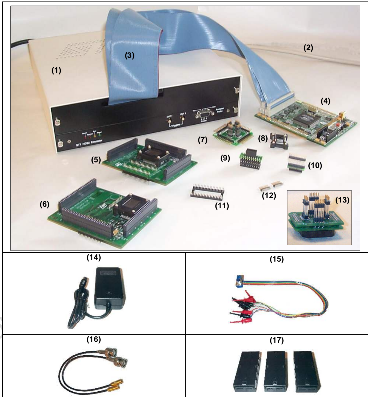
Figure 2: Main components of ST7MDTU2-EMU2B emulator kit
