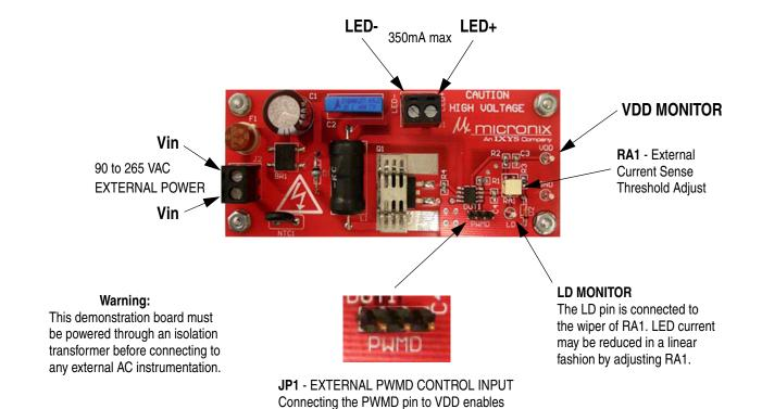
the converter. Applying a PWM TTL signal between the PWMD pin and GND adjusts the average output current to the LEDs according
