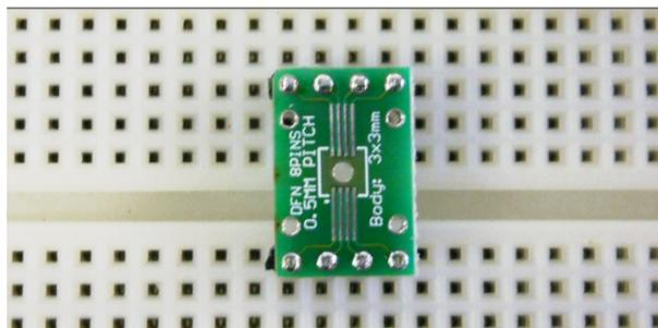
This product is an DFN to DIP adapter with a twist. These have our patented "ez" technology which means that soldering the surface mount component is simple, and as with all of our "ez" boards, we are the only company with a patented solution for easily soldering surface mount parts. Included in the package are two .5mm pitch adapter boards for 8 leads and a row of headers to use the boards with a breadboard.
