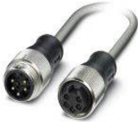
Bus system cable, DeviceNet, 5-position, PUR halogen-free, Gray RAL 7001, Plug straight 7/8"-16UNF, on Socket straight 7/8"-16UNF, Cable length: 15 m
